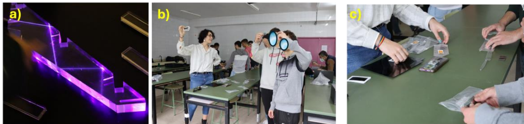
Figure 1. Performing experiments related to optical communications and polarization. a) plastic piece employed for refraction experiments, b) students using lineal polarizers and c) set of elements for the polarization experience
