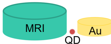
Figure 1. Scheme of one of the analyzed dimer configurations. In this case, the dimer corresponds to a hybrid nanostructure combining a moderate refractive index and a metallic nanoparticle.
