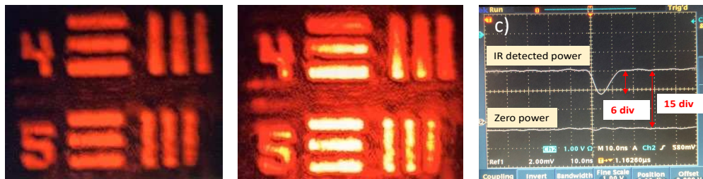
Figure 2. a) Upconverted image in CW. b) Upconverted image in synchronized pulse mode. c) Quantum Efficiency QE = 0.4 , representing a 98% power conversion efficiency.
